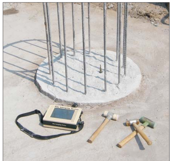
Integrity tester PIT Collector von Pile Dynamics Inc.
